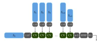
Figure 8.1: Schematic of KangarooTwelve for ||S|| > B, with arrows denoting calls to *F*.
