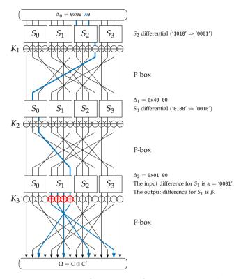
Figure 2.24: A 2-round trail ( $\Delta_0 \Rightarrow \Delta_1 \Rightarrow \Delta_2$ ) over a 3-round SPN leading to the recovery of 4 bits of  $K_3$  (highlighted in red).
