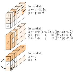
Figure 4.2: The SP-box applied to a column.
