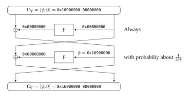
Figure 2.23: The 2-round iterative differential with a probability of  $\frac{1}{234}$ .
