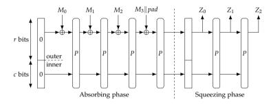
Figure 2.9: Basic sponge construction processing four message blocks  $M_0 \| \dots \| M_3$  and returning three blocks  $Z_0 \| Z_1 \| Z_2$ .
