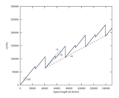
Figure 8.4: The number of cycles of KANGAROOTWELVE on an Intel Core i5-6500 (Skylake) as a function of the input message size.
