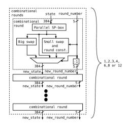
Figure 4.7: Combinational round in round-based architecture.
