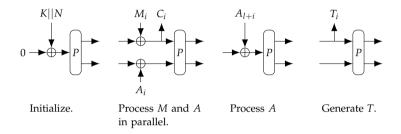
Figure 2.14: Another example of Authenticated Encryption sponge construction: FSW (Full-state SpongeWRAP, simplified).
