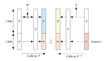
Figure 2.11: Targeting a preimage of Z by finding inner-collisions with a MITM approach.
