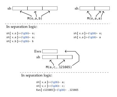
Figure 7.4: Aliasing and separation logic.
