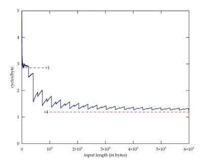
Figure 8.5: The number of cycles per byte of KANGAROOTWELVE on an Intel Core i5-6500 (Skylake) as a function of the input message size.
