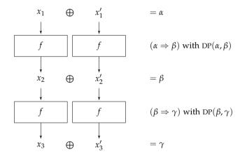
Figure 2.22: By combining two differentials  $(\alpha \Rightarrow \beta)$  and  $(\beta \Rightarrow \gamma)$ , we build a trail  $(\alpha \Rightarrow \beta \Rightarrow \gamma)$ .
