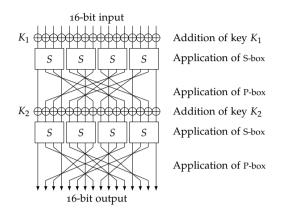
Figure 2.6: A 2-round 16-bit Substitution Permutation Network.
