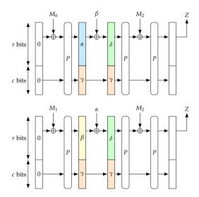
Figure 2.10: Exploiting inner-collisions to generate colliding outputs.
